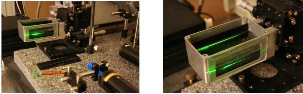
Fig. 12. Experimental set-up for detection of small size inclusions.
