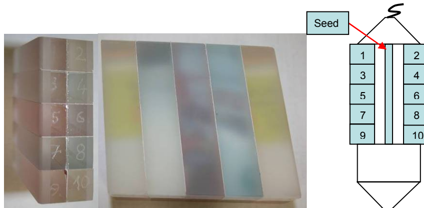
Fig. 3. Ten quartz crystal bars and their positions in the crystal.
